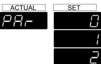
**PAr** - Parity bits of the serial interface
